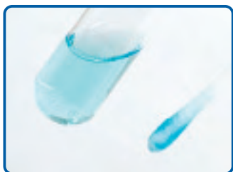
Traditional fiber swab elutes less specimen
