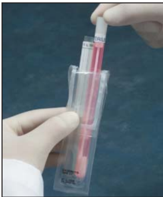
Close cap so swab is in contact with sponge in red tube
